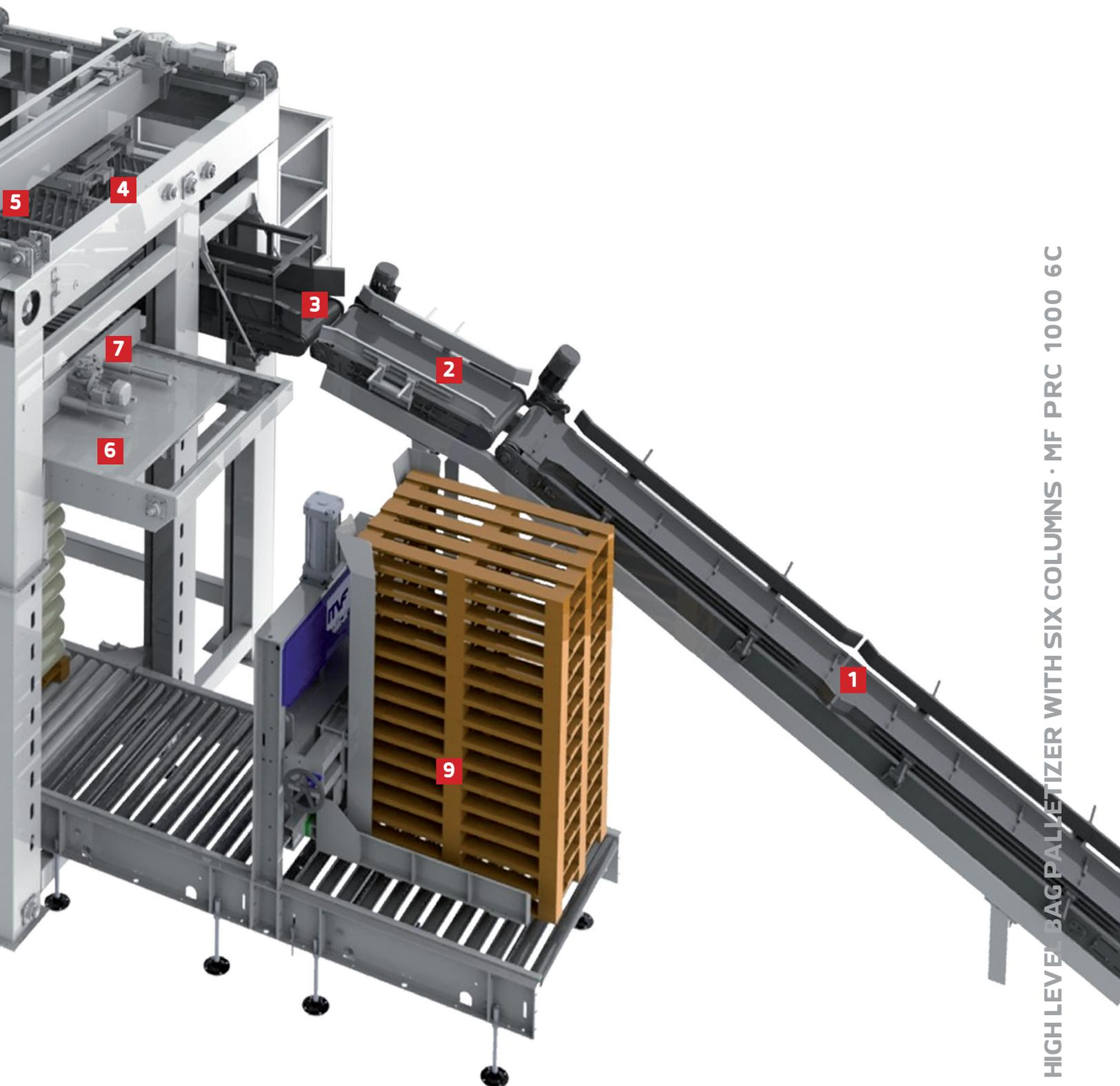
HIGH LEVEL BAG PALLETIZER WITH SIX COLUMNS · MF PRC 1000 6C
