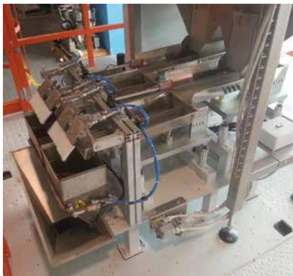
*In the case of packaging operations that do not involve particularly high volumes, products like those described up until this point can be dosed using one or more electronic scales equipped with Stainless Steel intake units with vibrating channels.*
